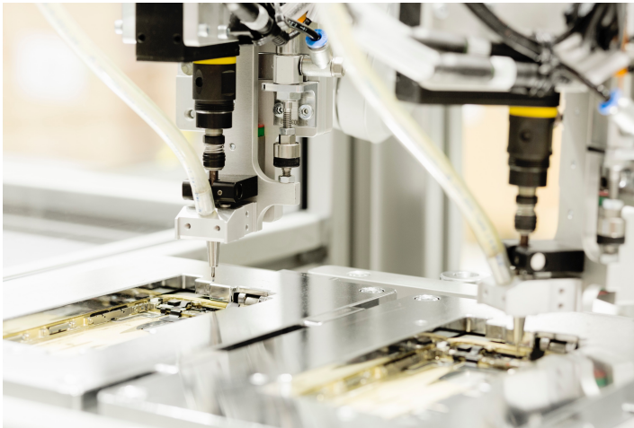
Dual-screw removal robots on the Liam line
