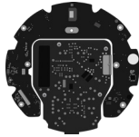
Power supply logic board
