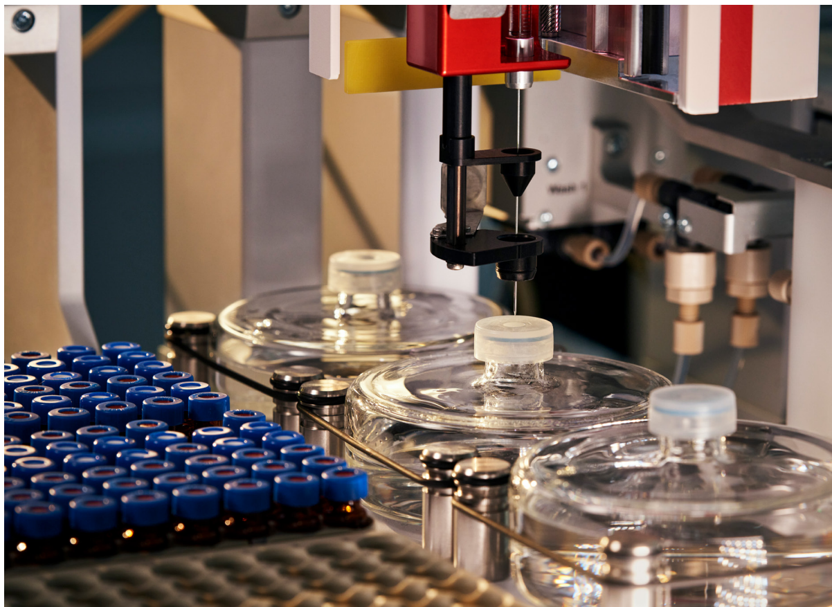
With equipment like this gas chromatography–mass spectrometry system, we evaluate materials for substances restricted in our Regulated Substances Specification, including VOCs.
