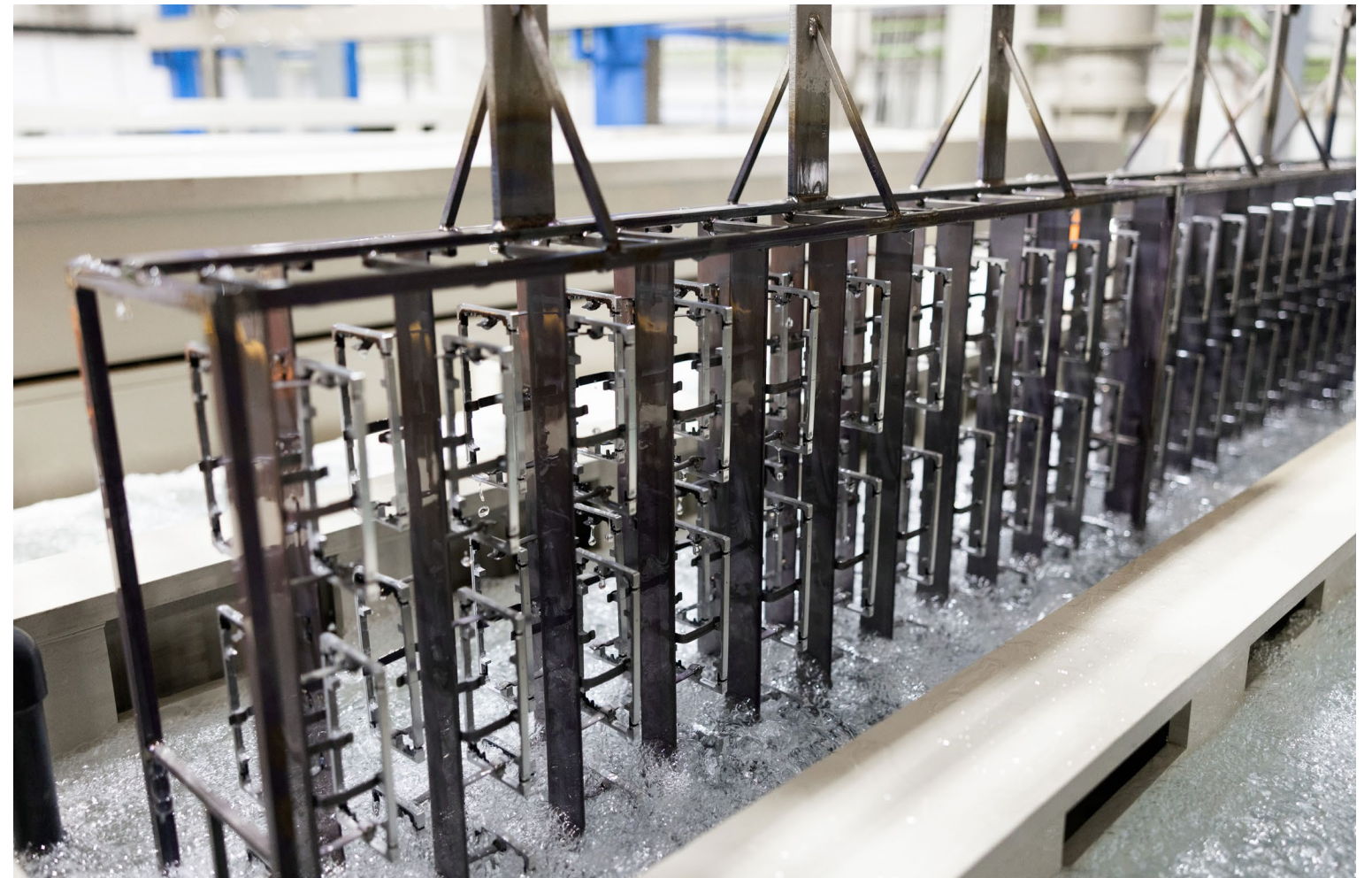
The aluminum anodizing process is typically water-intensive. In 2019, we launched a pilot to seek to eliminate hazardous discharge and increase water efficiency from anodizing. The cascade and counterflow rinsing processes, which helped retain 75 to 85 percent of the water used during metal finishing, could save millions of gallons of freshwater annually when applied at scale.
